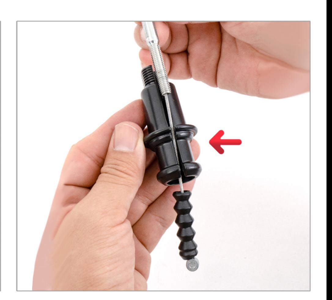
Turn clockwise to insert the cable and keep around 1cm threaded part out of the black housing. Turn rubber winder cap clockwise onto the black housing.
