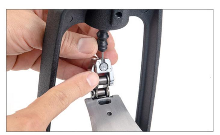
Relocate and tighten the screw in the slot.
